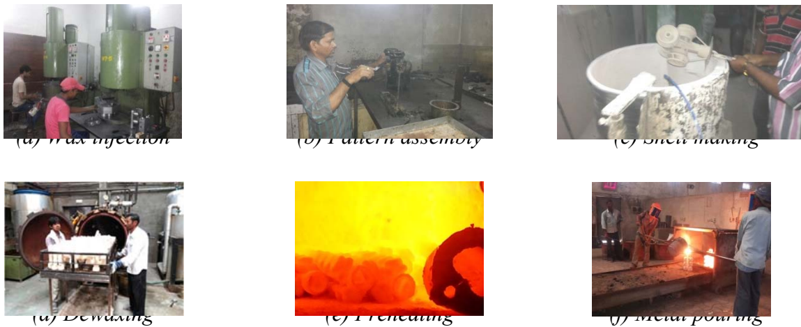
Figure 1: Investment casting process
