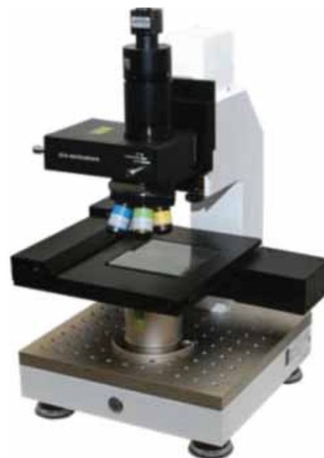
Fig. 11: 3D Microscope (Zata 20) used for surface inspection.
