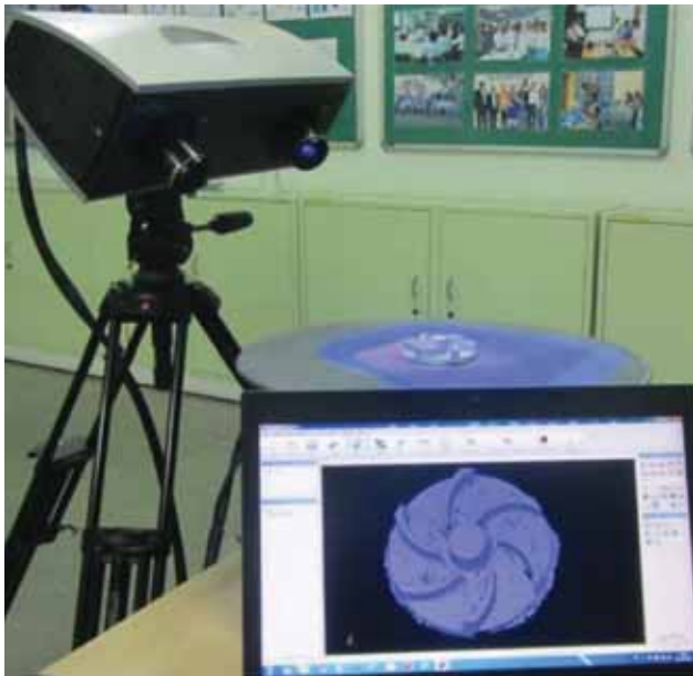
Fig. 9 : 3D scanning of impeller casting.
